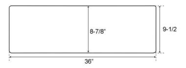
Dimensions of fixture are nominal and may vary within the range of tolerances established by ANSI Standard A112.19.2. Dimensions and specifications subject to change without notice.
